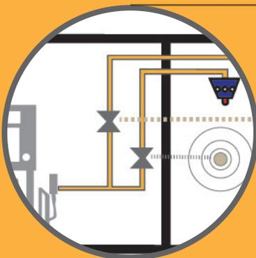
*Unlike the preaction systems, the piping is pressurised with downstream air instead of with water.*
