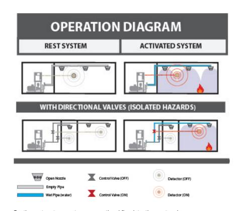
For the system to operate, a conventional fire detection system is necessary.
