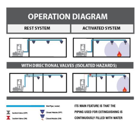
It stays filled with pressurised water until the automatic activation of the nozzle, which allows immediate action against the outbreak at the moment the fire is detected. The working pressure in the water line is 11-15 bar for ordinary hazards and 25-30 bar for special hazards.
